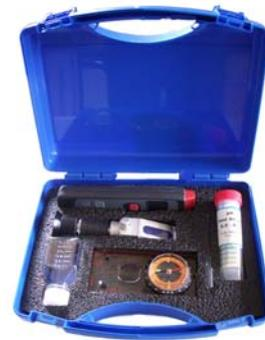
**During periodic routine maintenance**, the performance of the system is measured by taking temperatures at the top and bottom of the solar plate collector together with the inlet and outlet of the hot water storage tank, using the Mini Infra Red Thermometer.
