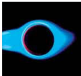
High flame temperature through cyclone swirl
