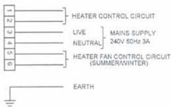
The mains supply for the POWRTROL may be taken from the heater control panel or from a separate supply. In either case there must be a facility to allow for complete electrical isolation of the unit.
