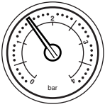
Fig. 19 Normal Pressure (operating)
