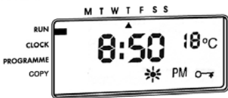
Display 1 - Shows current time and target temperature
