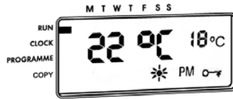
Display 2 - Shows current and target temperature
