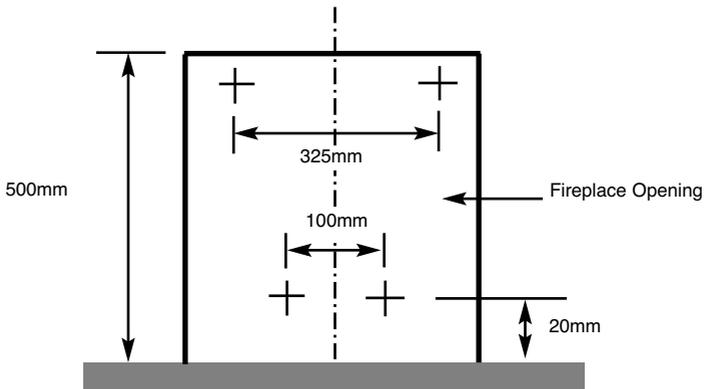
Fit the wallplugs provided and screw the fixing eyes securely into the rear of the fire opening. If the clearance at the rear of the fire is at the minimum specified for a precast flue application, it may be necessary to bend over the lower fixing eyes after screwing them fully in to the rear of a pre-cast starter block.
