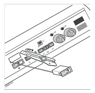
An optional flue gas thermometer may be fitted on the front of the control panel.
