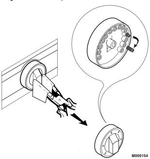
A factory-set stop limits the maximum temperature to 75 °C. To move the stop, proceed as follows:
