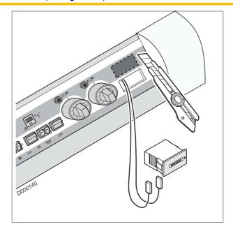
One or two optional hour run meters (stage 1 and 2) may be fitted on the front of the control panel. To do so:
