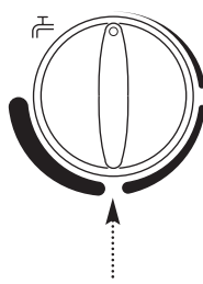
Domestic Hot Water Temperature Control
