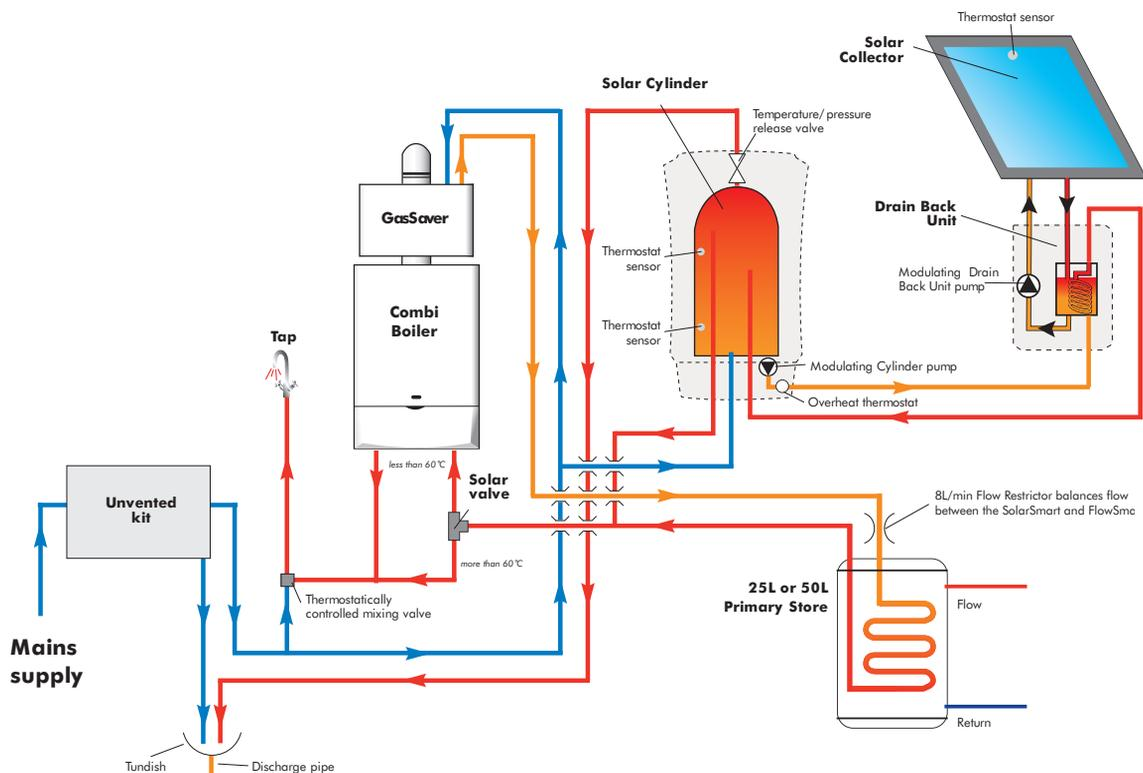
**NOTE:** In order to maintain good flow rates it is essential to have a supply of over 20L/min with a pressure above 2.5 bar (static), otherwise the flow rate out of the system will be reduced. This will also depend upon pipe layout and size.
